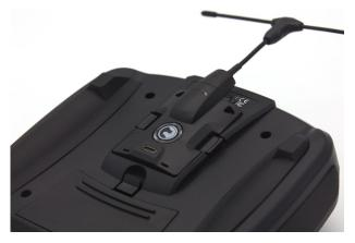
JR bay with installed TBS CROSSFIRE module
