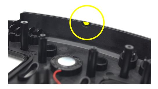
Feed the antenna wire around the internal PCB antenna and place the new SMA connector with the included washers in the hole, re-assemble the radio and tighten the nut down.
