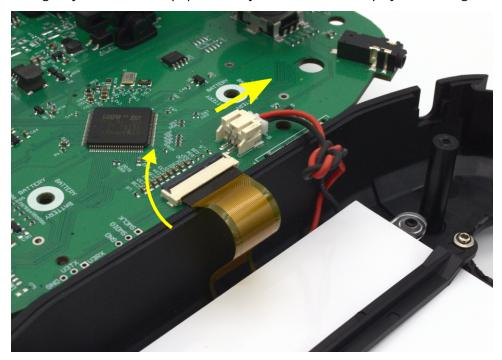
The gimbal support pegs are inserted on the mainboard holes and easily pulled out. Insert the new gimbal(s) and re-assemble the radio. Flap the PCB over the front shell, slide the switches into their holes, place the trim switches with a tweezer and gently push it in. Install the screws holding the PCB.
