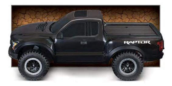
**MODEL 58094-1**: Fully-assembled, Ready-To-Race®, with TQ™ 2.4GHz radio, 4-amp DC Peak Detecting Fast Charger, Waterproof Electronics with XL-5 Electronic Speed Control and ProGraphix® painted body.
